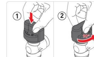
The valve may only be opened by pressing the handle [1] and subsequently turning it by 90° [2].
