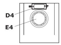
Once you have chosen the cleaning cycle to clean the cooking chamber, all you need to do is to confirm it by pressing the program knob **E4**.
